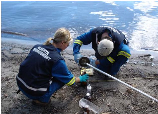
Alberta Environment and Parks staff collect river water samples and test them for nutrients, metals, bacteria, pesticides, etc.
