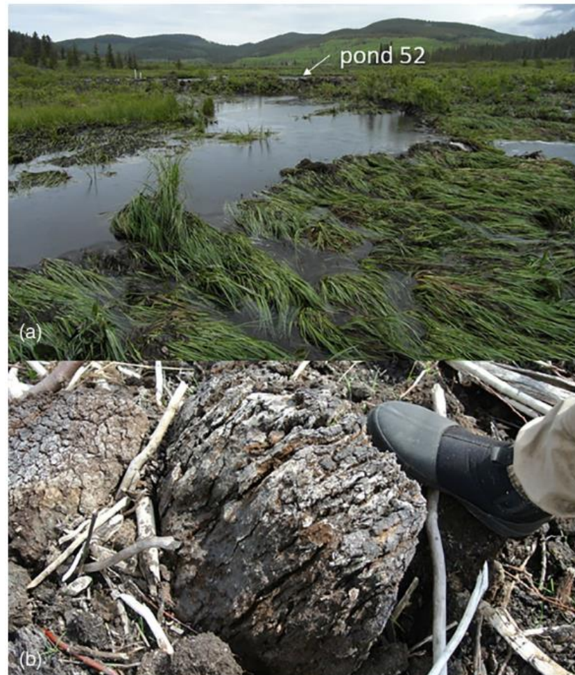
FIGURE 6 Photographs of: (a) Pond 52 after the flood event (June 30, 2013) showing flattened vegetation indicating outburst flood from pond 53 water flowed overtop of it, leaving the dam reasonably intact and the pond storing water; and (b) blocks of peat sheared from just below the dam breach at pond 53 found approximately 50 m downstream
