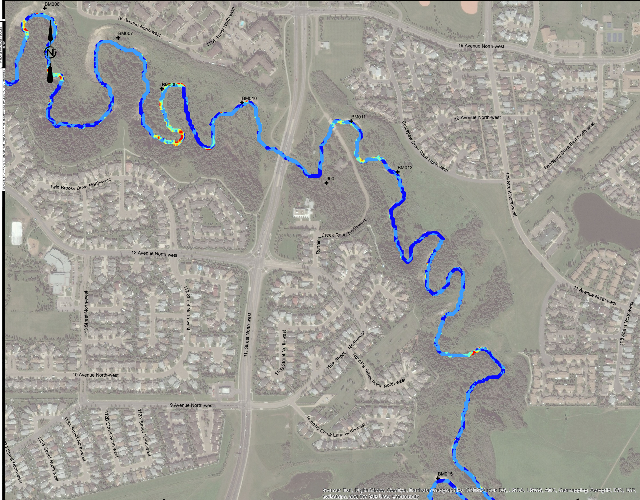
FIGURE No. D-20 BLACKMUD/WHITEMUD CREEK WATERSHED MANAGEMENT STUDY FUTURE DEVELOPMENT DISCHARGE RATE 3.0 L/s/ha RATIO TO EXISTING - 100 YEAR FLOOD VELOCITY AE PROJECT No. 2016-3785 SCALE 1:5,000 APPROVED DATE 2017 MARCH REV DESCRIPTION ISSUED FOR REPORT
