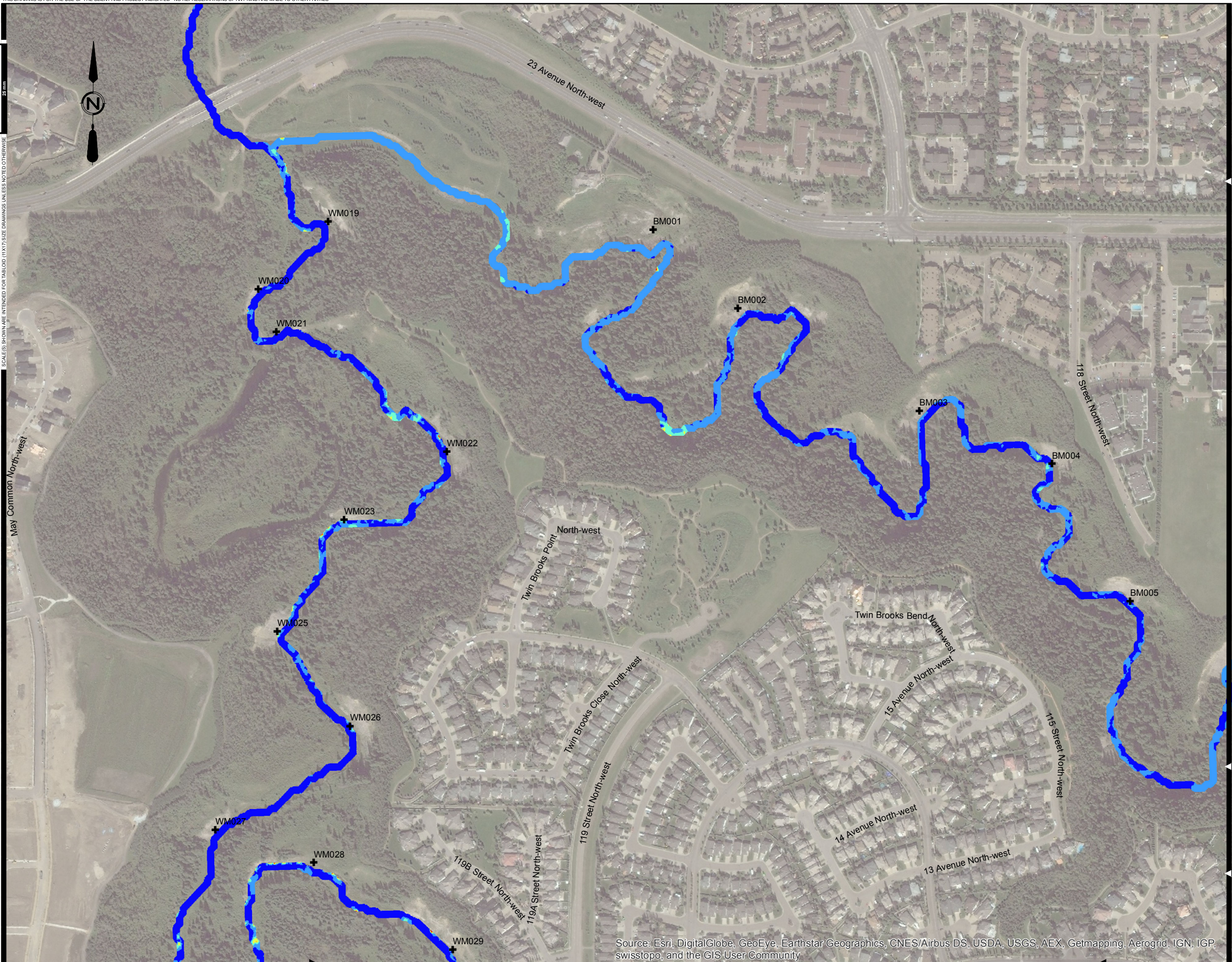
FIGURE No. D-5 BLACKMUD/WHITEMUD CREEK WATERSHED MANAGEMENT STUDY FUTURE DEVELOPMENT DISCHARGE RATE 1.5 L/s/ha RATIO TO EXISTING - 100 YEAR FLOOD VELOCITY AE PROJECT No. 2016-3785 SCALE 1:5,000 APPROVED DATE 2017 MARCH REV DESCRIPTION ISSUED FOR REPORT
