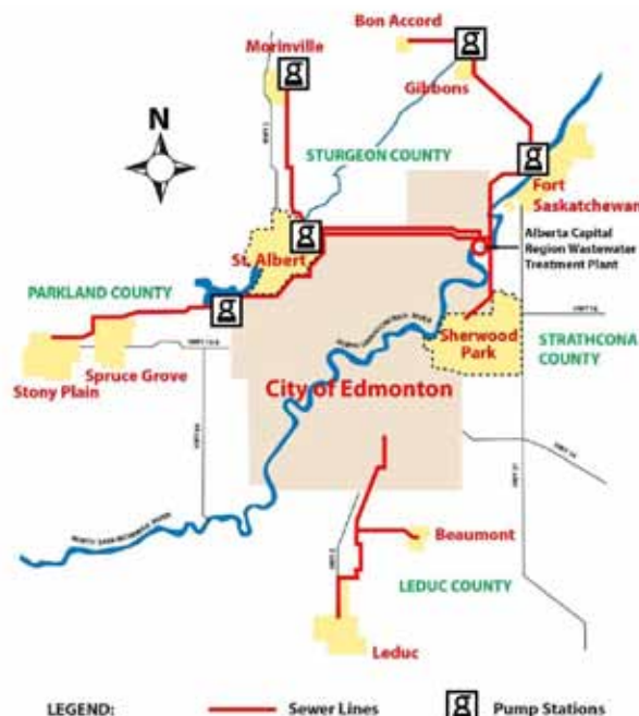
Figure 15. Alberta Capital Region Wastewater Commission transmission network. Image from Alberta Capital Region Wastewater Commission (2012).
