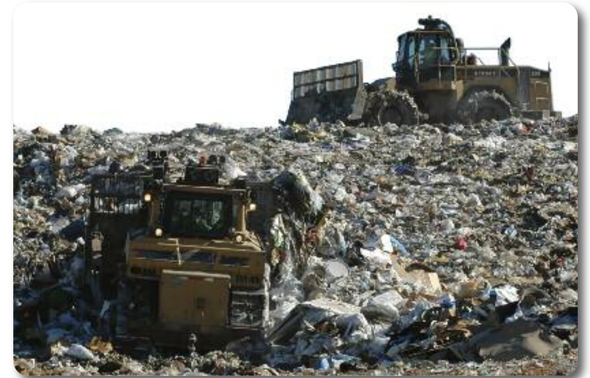
Facilities such as landfills and large confined feeding operations must be placed carefully on the landscape to avoid contamination of groundwater supplies through the infiltration of leachate.
