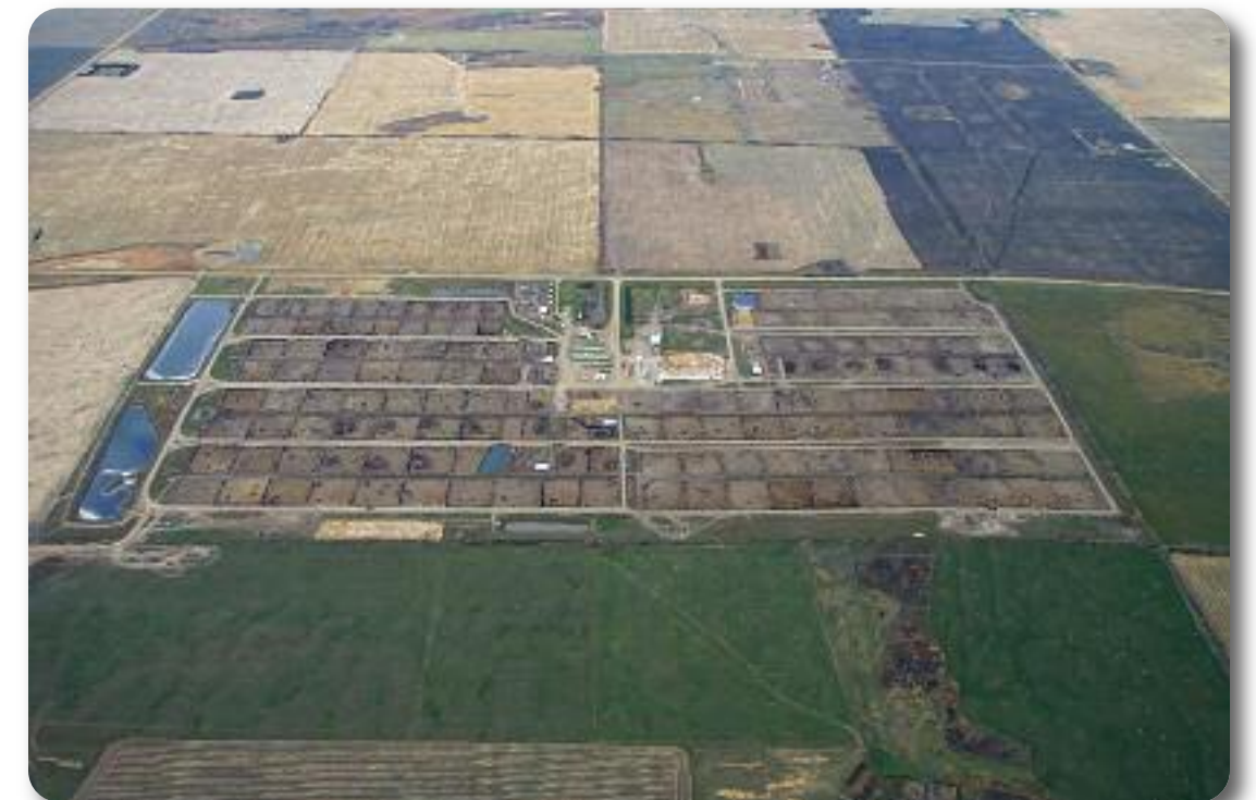
Facilities such as landfills and large confined feeding operations must be placed carefully on the landscape to avoid contamination of groundwater supplies through the infiltration of leachate.
