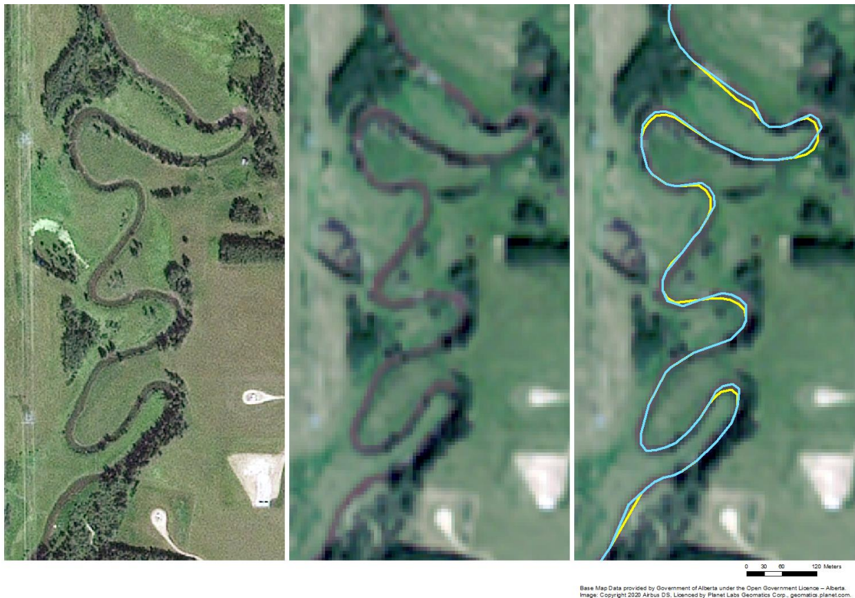
Figure 5. Example of the spatial inaccuracies associated with stream boundaries, where the location of the stream centre line does not match the actual location of the stream and exceeds the 5 m accuracy tolerance in the SPOT imagery. In this example, the yellow lines represent the location of the streamline from the provincial data and the blue line represents the manually edited location of the new stream centre line.
