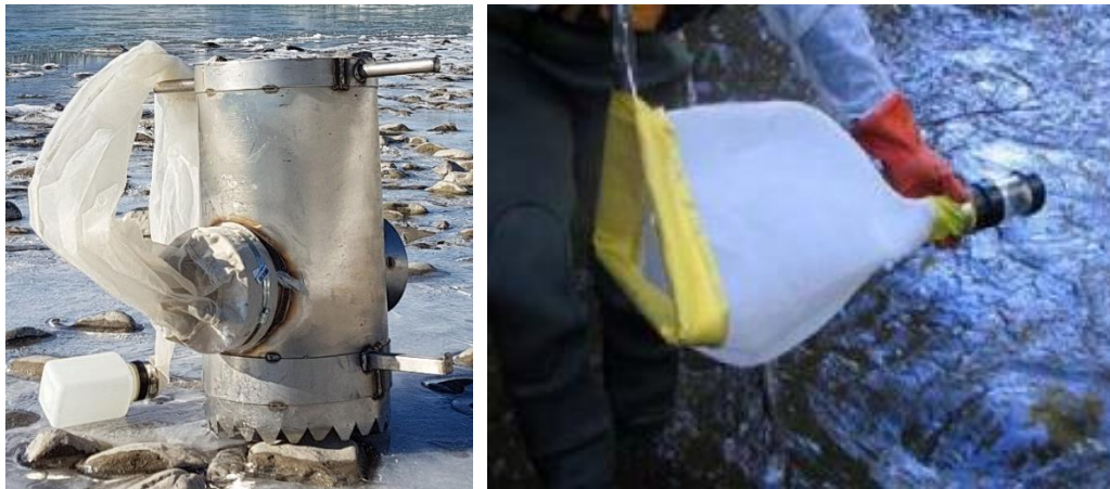
Figure 15. Neil cylinder (left) and kick-net used in CABIN sampling protocol (right).
