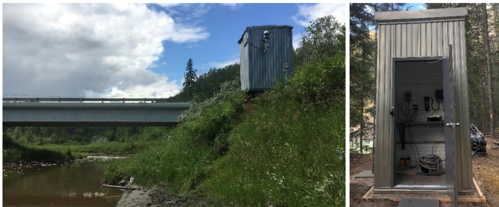
Figure 5. Photos of hydrometric stations deployed nearby Strawberry Creek (left) and the Siffleur River (right).
