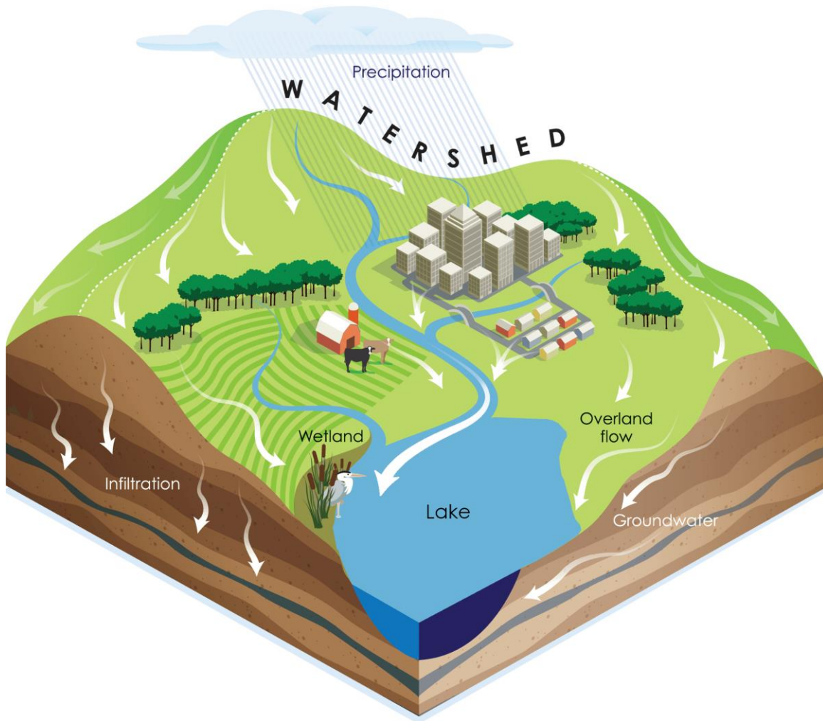
Figure 1. A Watershed. The white arrows show how water can flow through the watershed and into the lake. The white dotted outline is the boundary of the watershed. Outside the boundary, the water does not flow toward the lake.
