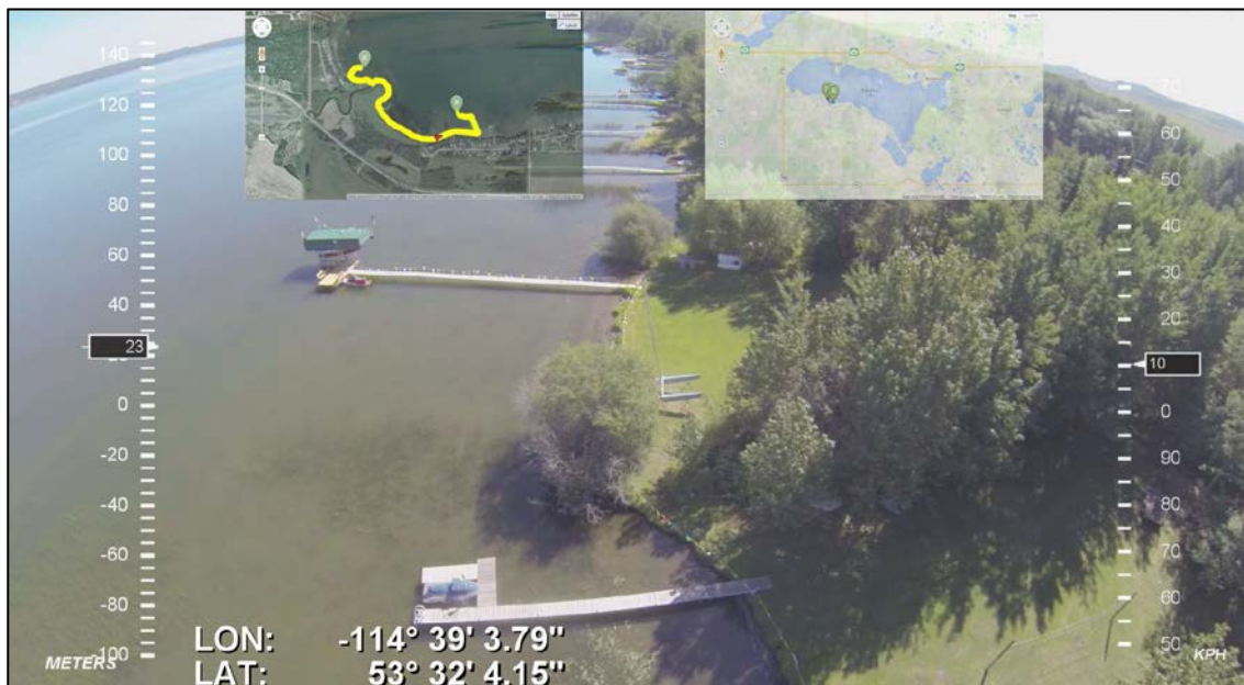
Figure 5 Screen shot of post-processed video footage. The footage now includes spatial data overlaid. The bar-scale on the left is measured in meters above the launch height. The bar-scale on the right is speed measured in kilometers per hour.
